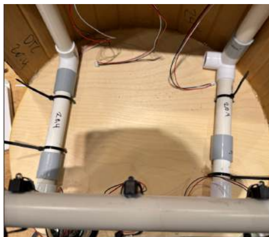
Figure 24. The zip ties attached to the frame
