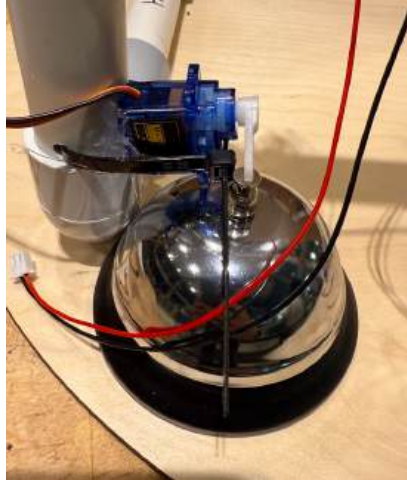
Figure 25. Servo ziptied to the leg of the frame and hot glued.
